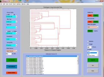
Cluster analysis provides insight into the chemical relationships between sample classes derived from the measurements of the **NoseChip**<sup>™</sup> sensor array.
