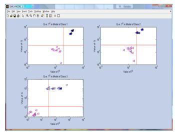
SIMCA is a supervised classification method for sensor data using Q and  $T^2$  statistics to construct boundaries for class identification.
