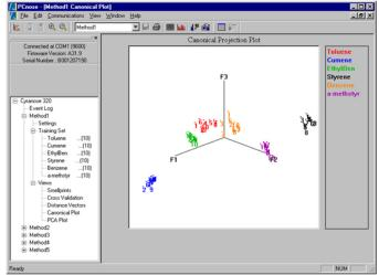
Discrimination results are visualized in 2D and 3D displays of the **smellprints**<sup>™</sup>, distance vectors, PCA and CDA scores for simple and complex data sets.
