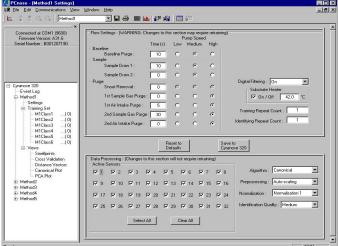
Operators have complete control over the flow rates and sampling durations, selection of chemical sensors (from 1 to 32), and data processing and analysis parameters.
