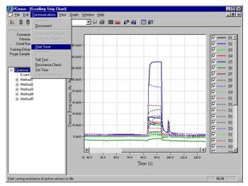
The scrolling strip chart provides visualization of the sensor response for all 32 chemical sensors for optimization of air sampling parameters and instrument settings.
