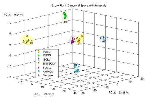
Air samples collected from outdoor sources can be distinguished by the **type of odor**, such as, wastewater treatment, composting, landfills and rendering operations. This is due to the difference in chemical composition of the odors measured with the **NoseChip**<sup>™</sup> sensor array.
